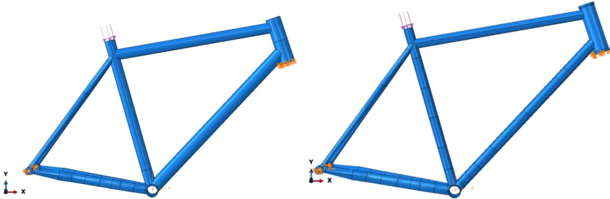
Figure 4. Loading and boundary constraints for both aluminum (left) and steel (right) models. The orange arrows represent boundary constraints
