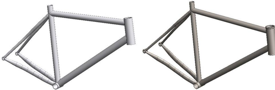
Figure 3. a) Aluminum frame shown on the left, b) steel frame shown in right. Note the use of cylindrical rear axle dropouts.
