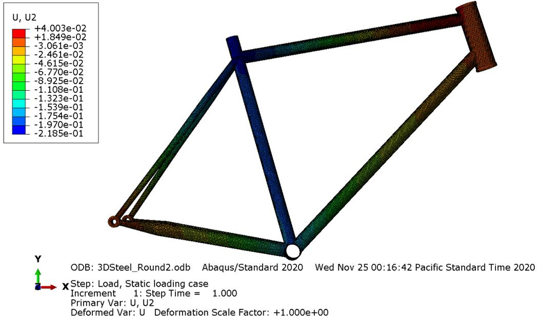
Figure 7. Side profile image of 3D steel model utilizing round 2, from Table 2, global seed sizes.
