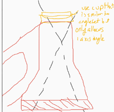
consider slackening influence by adding at the bottom Adjustment done on the lower cup instead of upper
