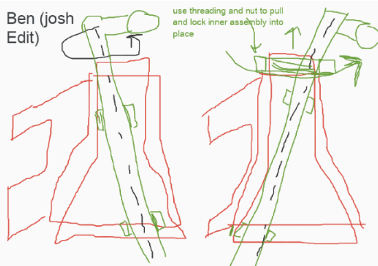
Rotating inner headtube assembly offering two positions
