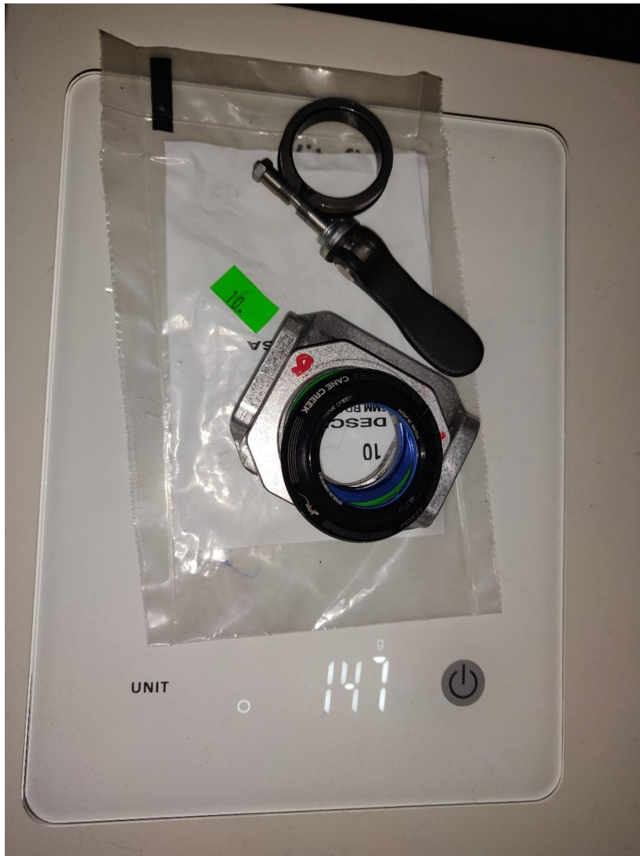
Figure 2. Top cup assembly including: top cup, top bearing housing, top bearing, dust cap, and compression ring.
