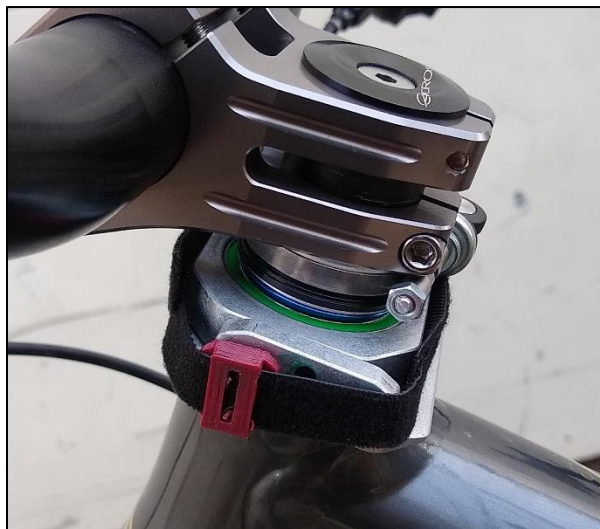
Figure 39: Pin retention system installed on the headset.
