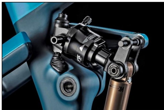
Figure 4a. Canyon ShapeShifter gas piston linkage interaction (Canyon).
