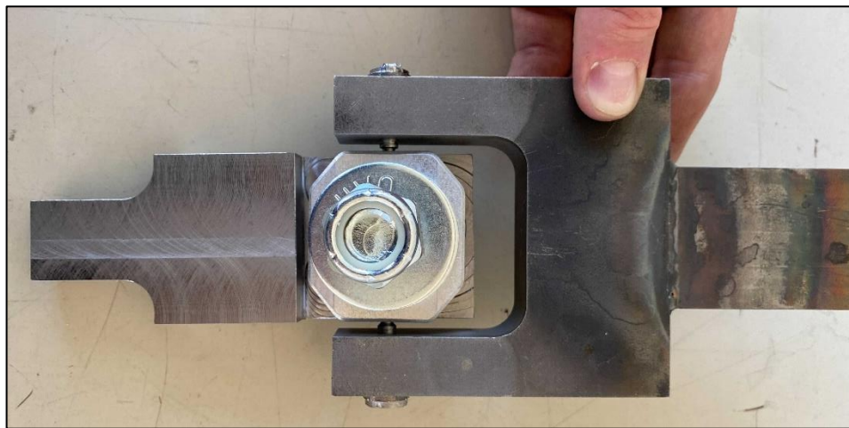
Figure 45: Assembled bearing housing test fixture.
