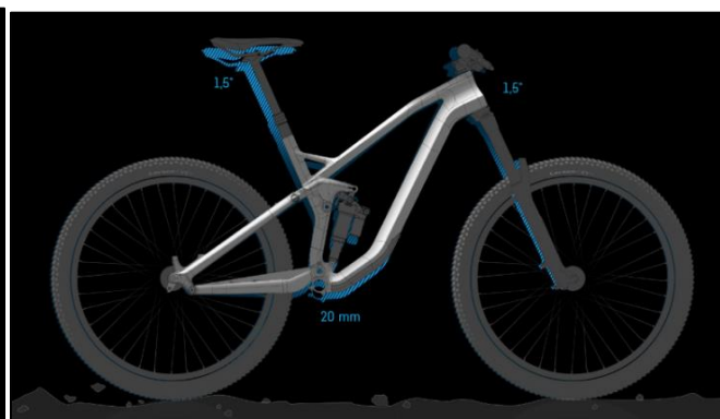
Figure 4b. Geometry alteration caused by activation of the ShapeShifter system (Canyon).
