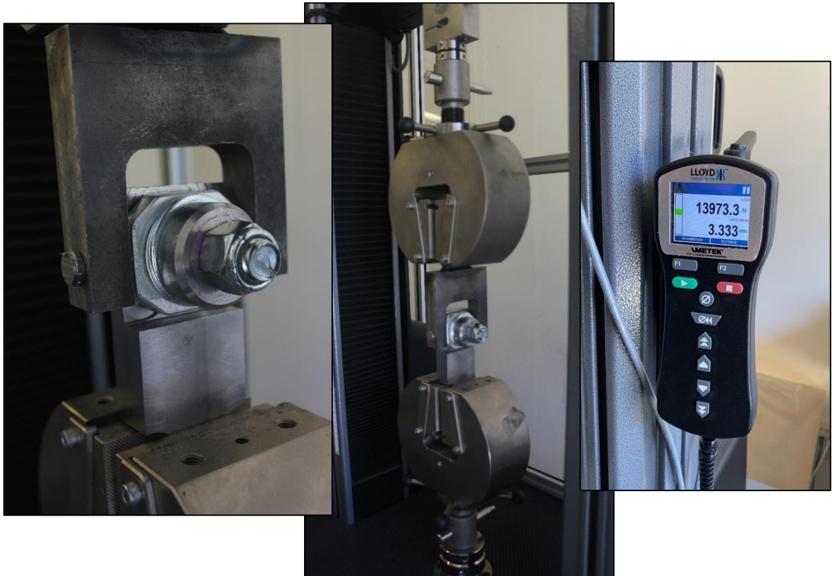
Figure 51: Images of Instron load test conducted on the Top Bearing Housing.
