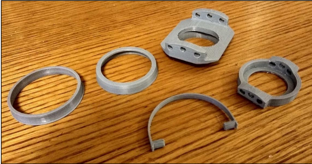
Figure 31. Assorted 3D printed parts as the structural prototype.
