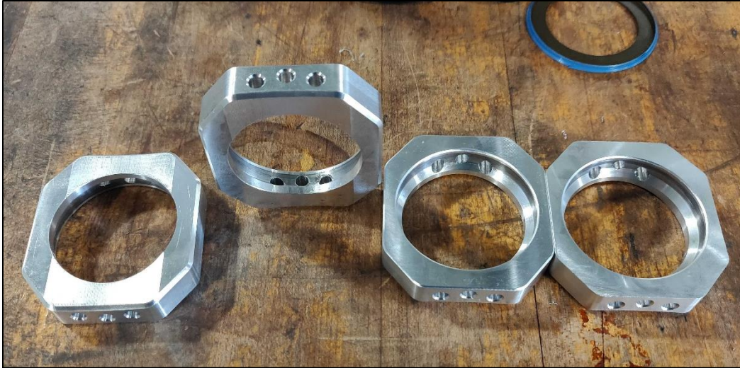
Figure 38: Completed top bearing housings.
